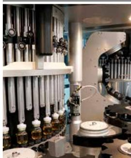
With our Bern site aiming to significantly boost production over the next several years, an innovative solution was needed to ensure all of the product could be inspected. Project Eagle answered the call. The project, which consisted of the implementation of fully automated inspection technology has boosted inspection rates from 35 vials per minute to 180 vials per minute, ensuring manufacturing operations can keep up with future demand.
