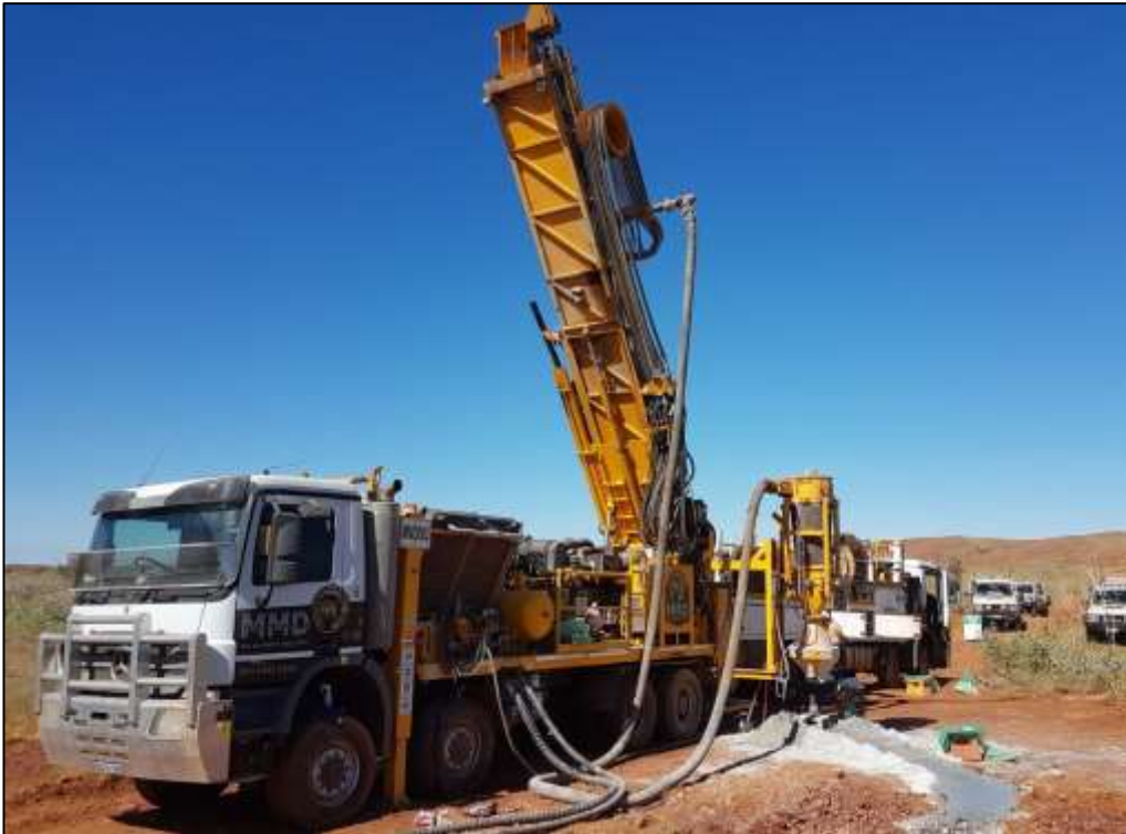
Figure 7: Reverse Circulation (RC) drill rig operating at the Fuego prospect, Croydon Project.
