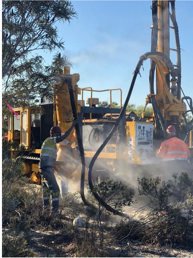
Commencement of 32 Hole Air-Core Drilling at Beharra
