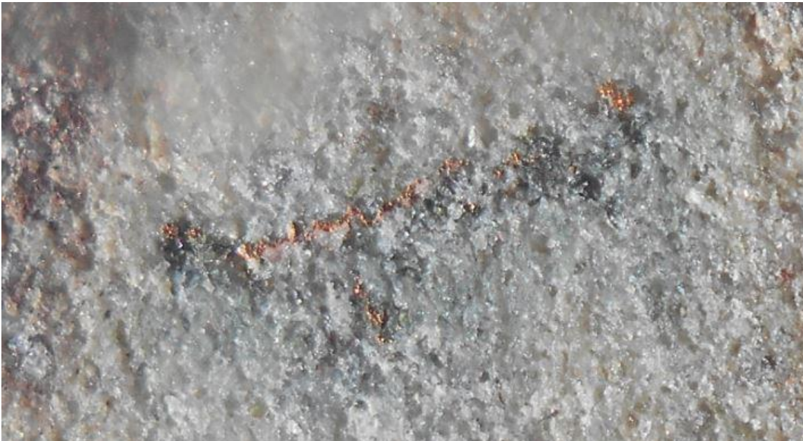
Figure 5: Small vein of native copper in sediments overlying the basement material.
