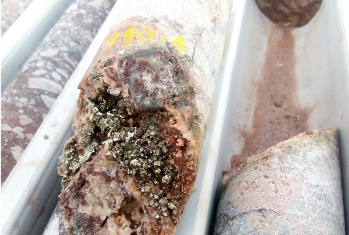
Figure 4: Highly altered basement material with open space pyrite vein.
