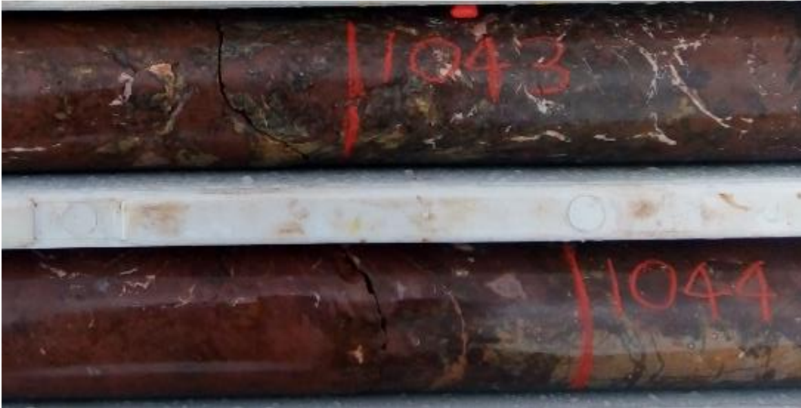
Figure 6: Red, earthy, hematitic ironstone encountered in HWDD03 at 1,043m.
