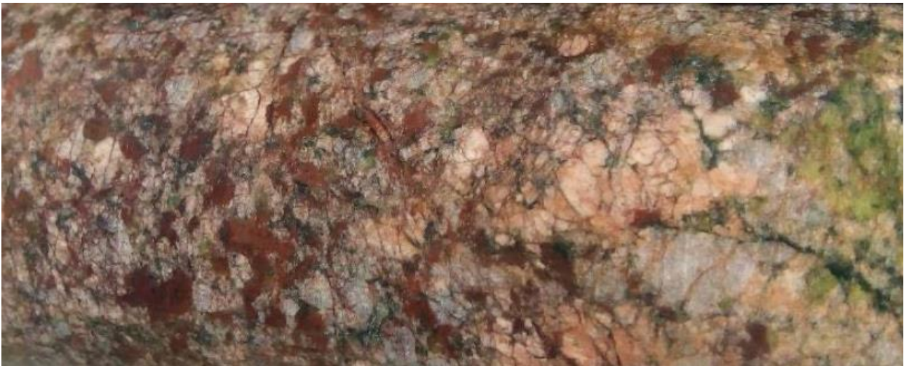
Figure 3: Coarse grained, altered granite encountered at 960m in HWDD02.
