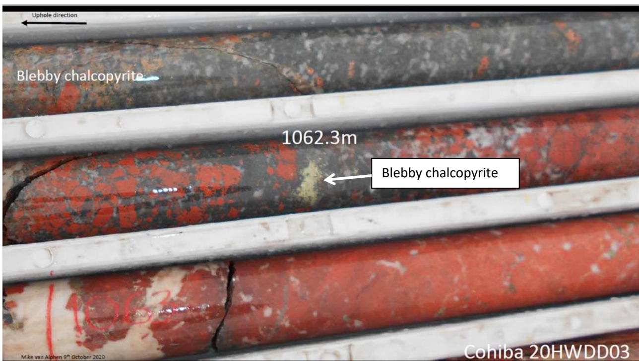
Figure 1: Earthy hematite + quartz + K-feldspar with blebby chalcopyrite (1062.3 m).
