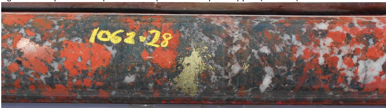
Figure 2: Close up of blebby chalcopyrite from Figure 1 (@1062.28m)
