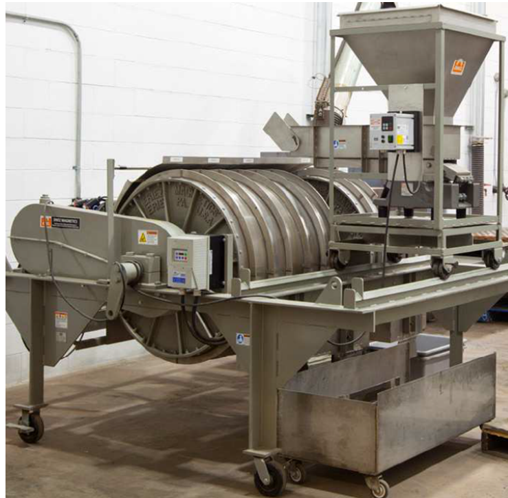
Figure 1 – Polimin pilot magnetic separation equipment used during some of the Yerbos Buenas tests
