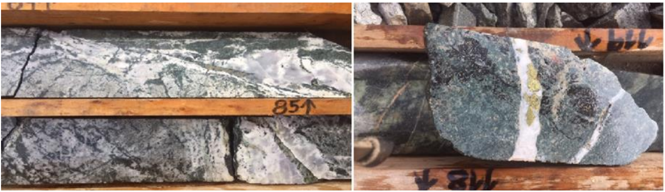
Figure 5 - Diamond core from hole ES-001 drilled into Induced Polarisation target. Samples 4513, interval 84-85m showing intense alteration and sample 4547, interval 118-119m showing visible chalcopryrite veining.
