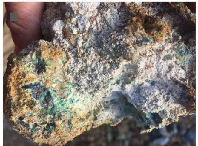
Figure 7- NW vein zone, quartz-albita-actinolite-clays-sericite-chalcopryrite (2.5% Cu, 1.3g/t Au) channel sample 311814
