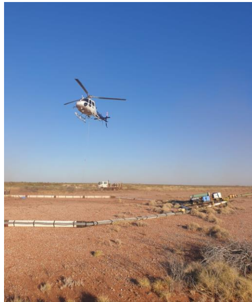
Image 3: SkyTEM begins HEM survey at West Wits' Mt Cecelia project in the Paterson Province
