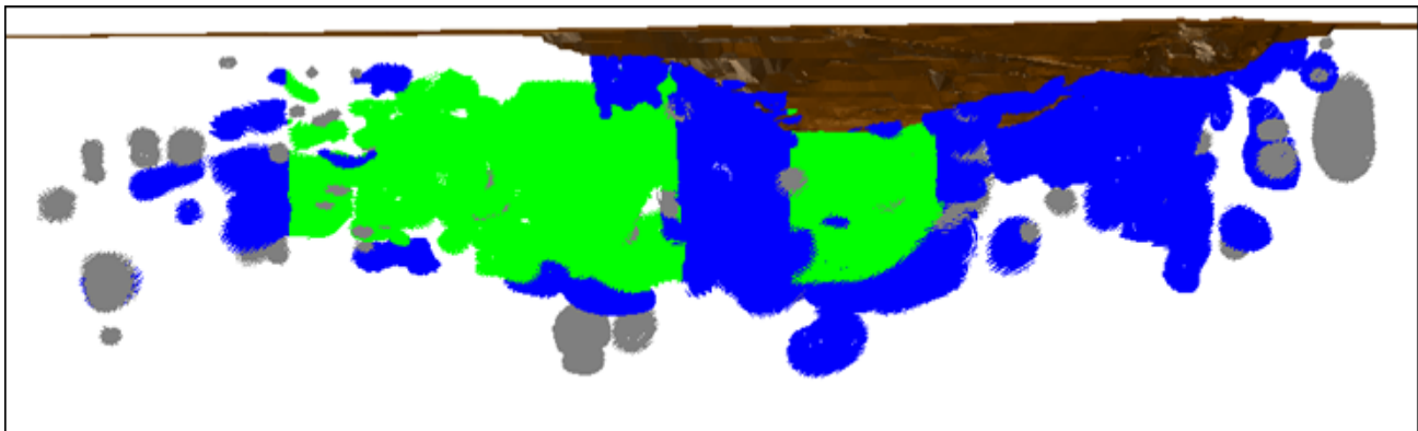
FIGURE 1. OBLIQUE VIEW (LOOKING WEST) DISPLAYING THE BLOCKMODEL CLASSIFICATION INDICATED (GREEN), INFERRED (BLUE) AND UNCLASSIFIED (GREY) BLOCKS.
