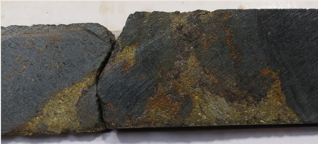
Figure 2: ¼ core sample of 10CHRCD005 from 230.5m showing chalcopyrite and pyrrhotite in gabbro
