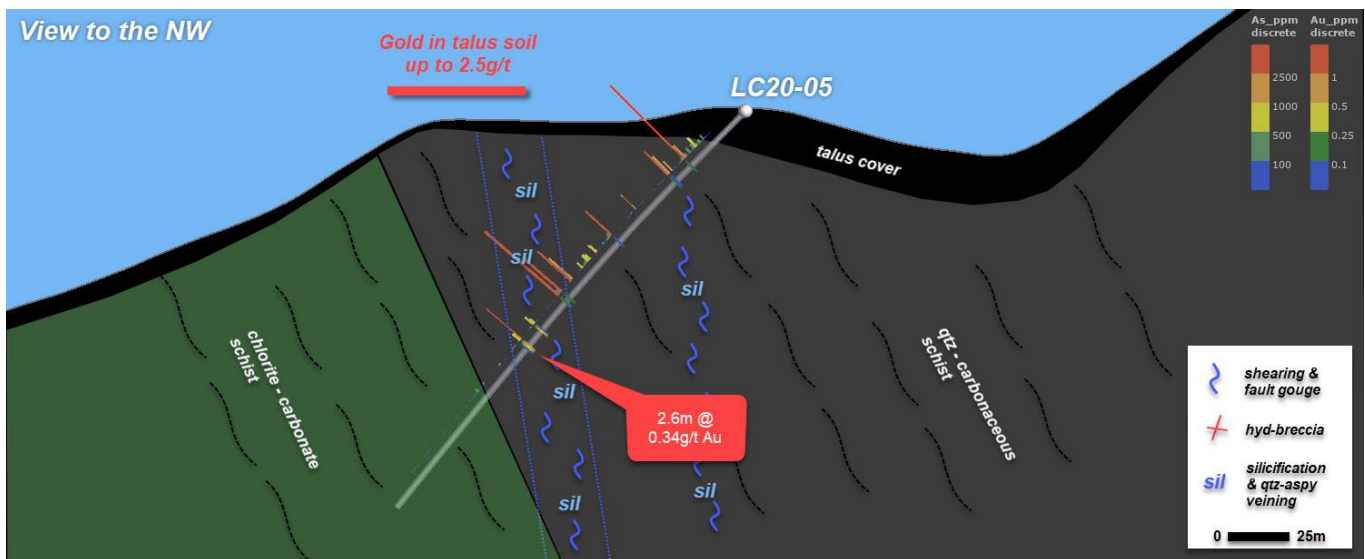
Figure 8: Cross-section for LC20-05 showing gold (drill trace) and arsenic (histogram) anomalism associated with zones of quartz-arsenopyrite veining and silicification below a mapped hydrothermal silica breccia body at surface.
