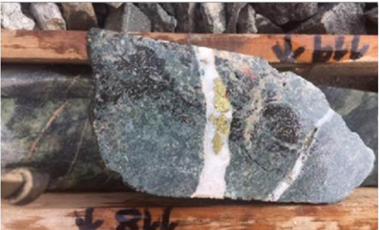
Figure 5 - Diamond core from hole ES-001 drilled into Induced Polarisation target. Sample 4547, interval 118-119m showing visible chalcopyrite ( copper sulphide) veining.
