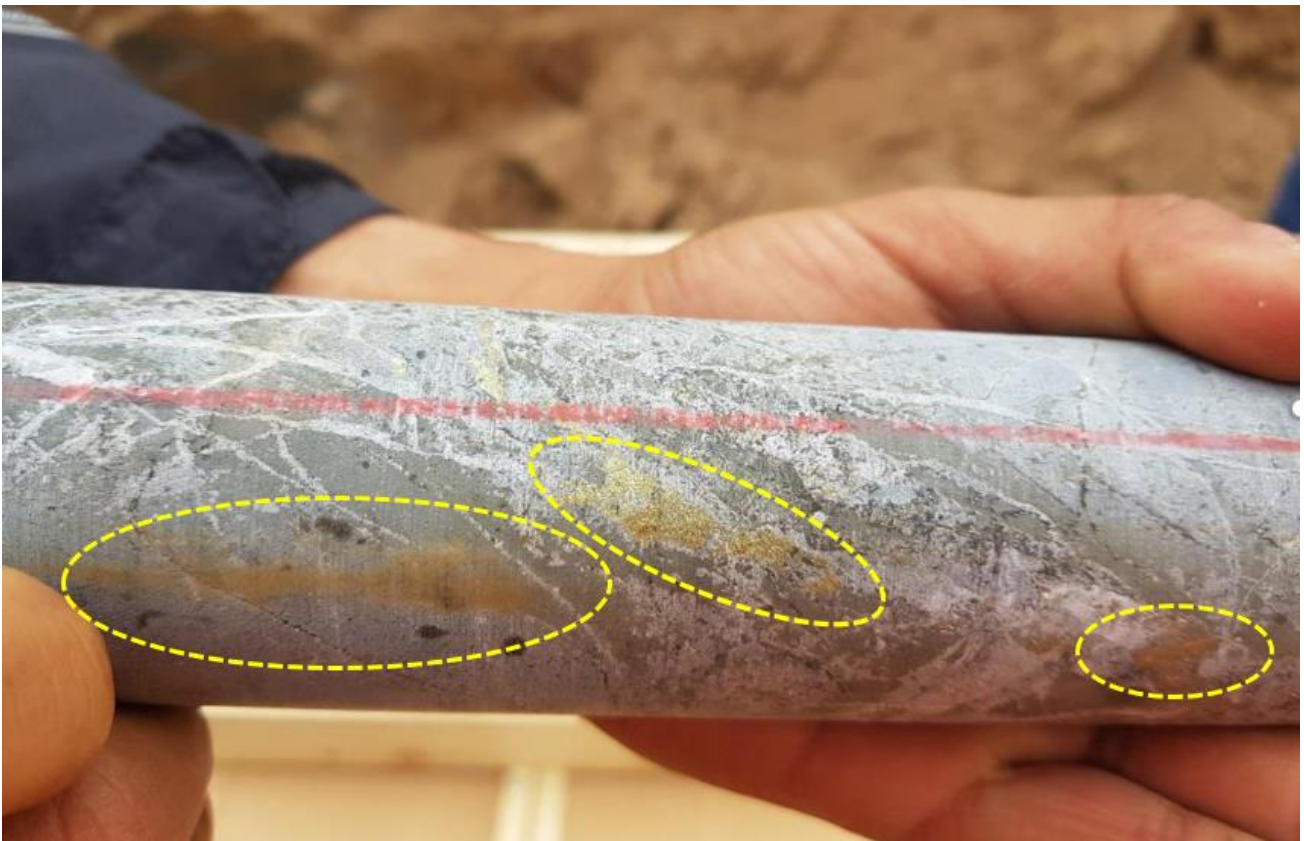
Figure 6 – Diamond core from hole ES-001 drilled into Induced Polarisation target. Sample is 4520, interval 91-92m showing visible chalcopyrite (copper sulphide) veining circled in yellow.
