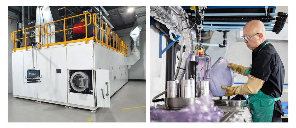
The XTclave is an **advanced composite materials curing and consolidation technology**, that uses ultra-high isostatic pressure at elevated temperatures
