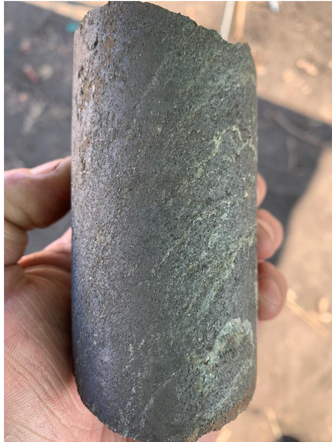
Figure 8 BEKD01 52.5m –Massive Magnetite (black) with narrow layers of Calc-Silicate host rock (white and green)
