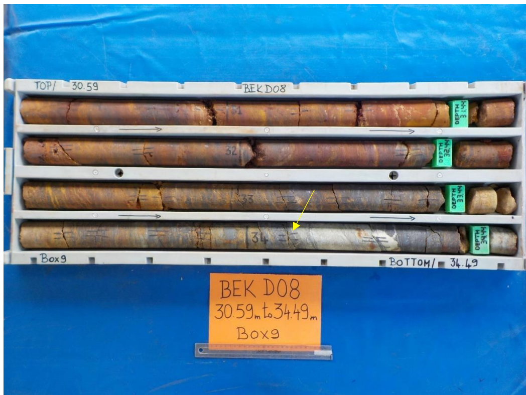
Figure 11 Massive Magnetite with some Hematite/Goethite due to weathering (BEKD08 29-34m) note that the yellow arrows mark the start and finish of the massive magnetite-hematite-goethite
