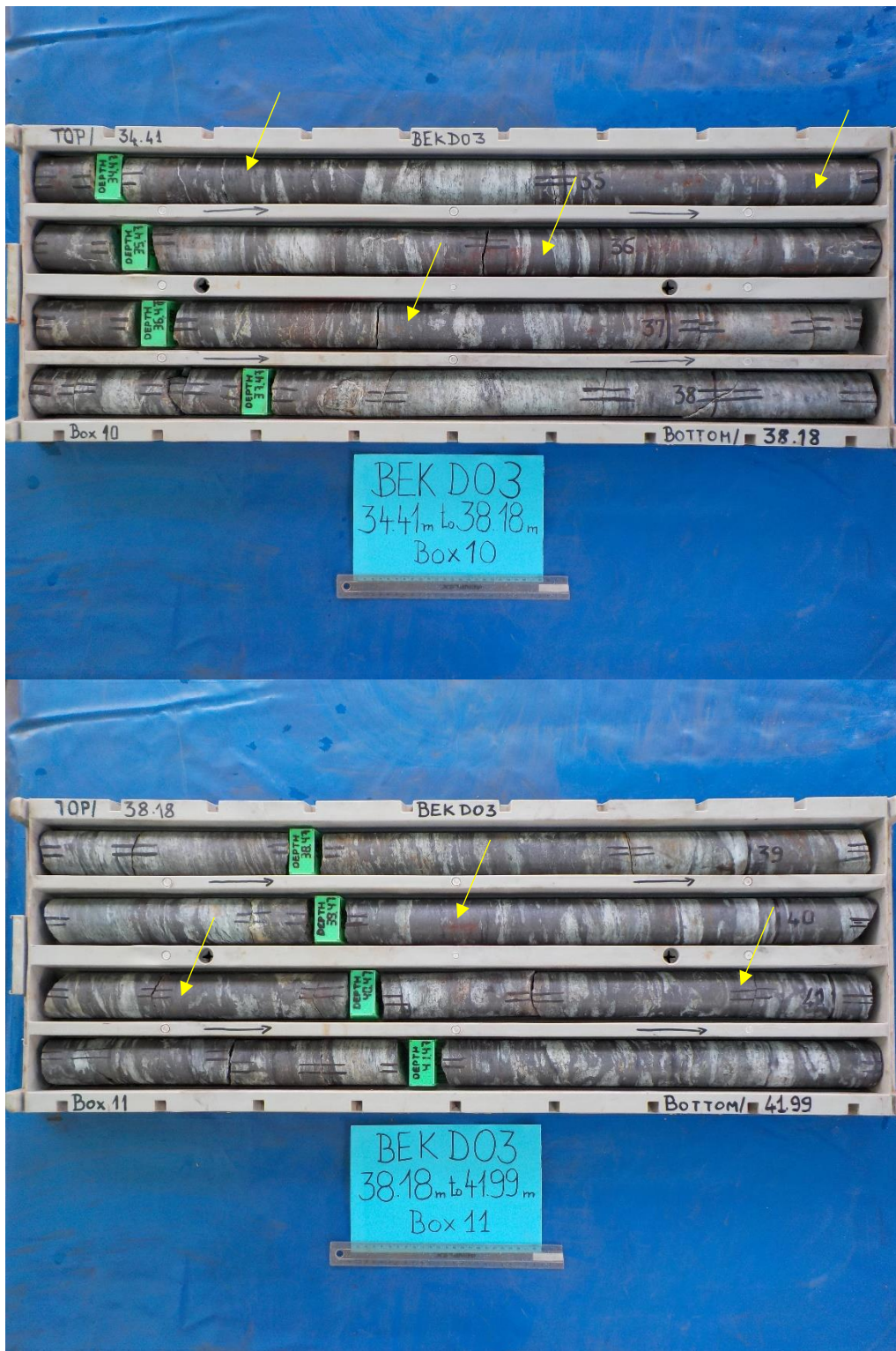
Figure 10 BEKD3 34-42m; Massive Magnetite layers (black, several highlighted by yellow arrows) within Calc-Silicate and Gneiss (white)
