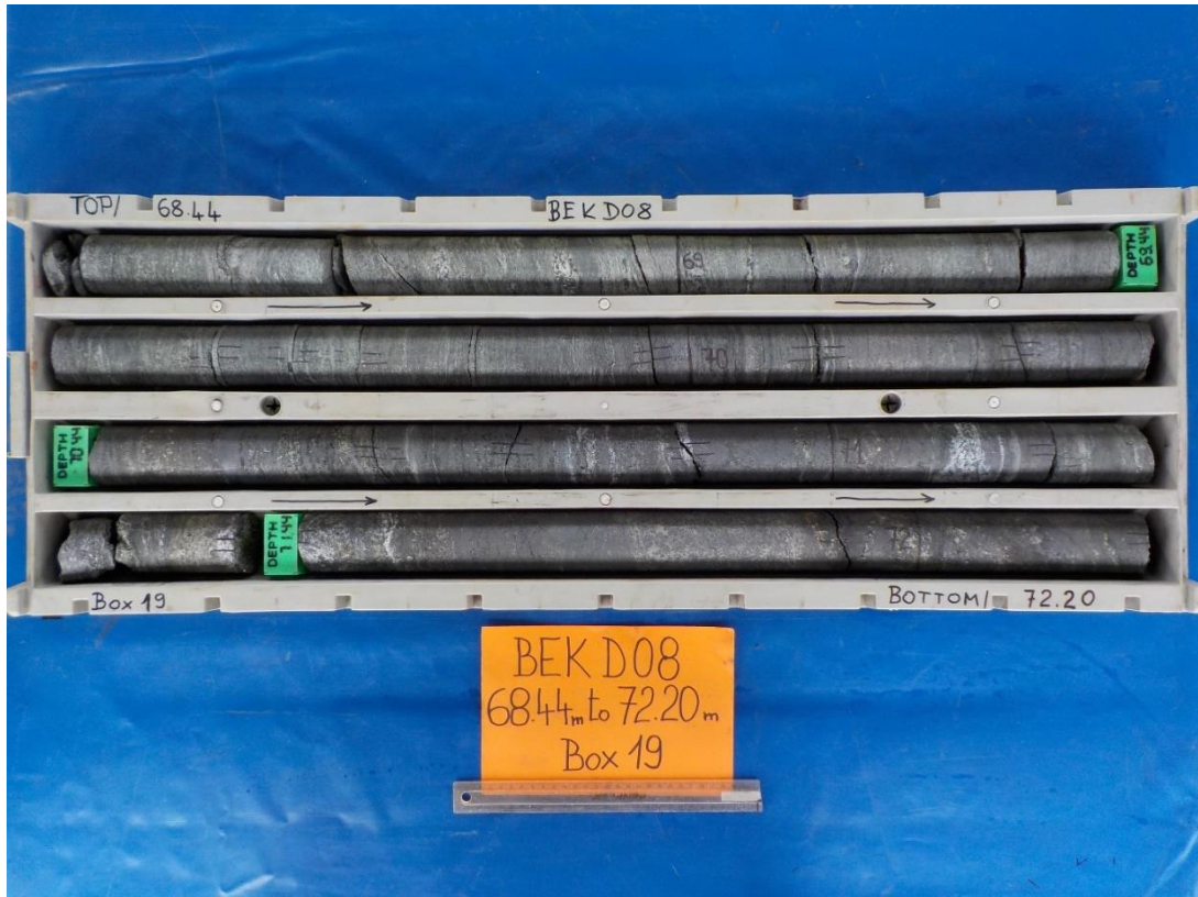
Figure 12 BEKD08 70.4-72.2m; Massive Magnetite (black) with streaks of Gneiss and Calc-Silicate (white)
