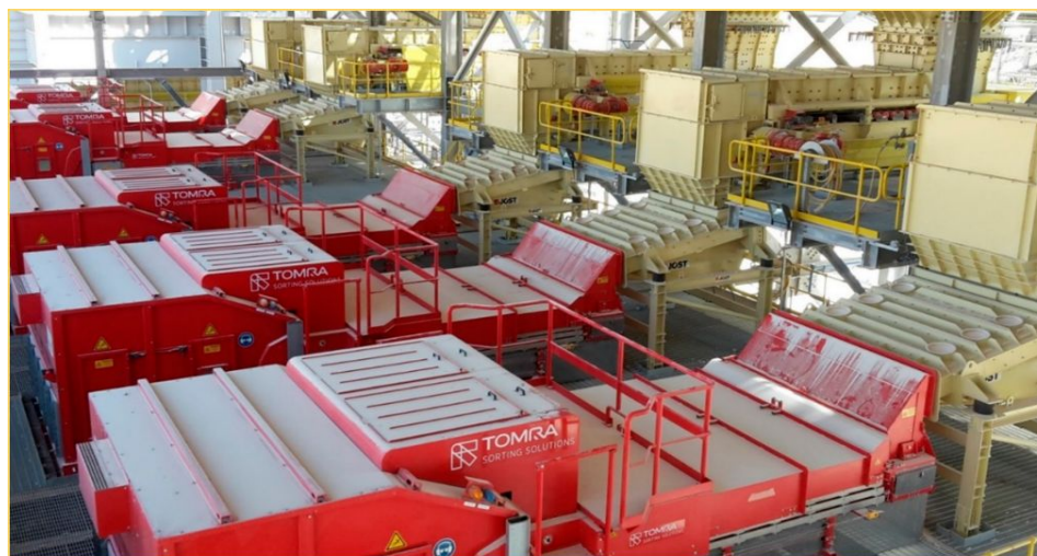
Nameplate capacity is the 1800 tons per hour XRT-based sorting plant at the Umm Wu'al phosphate mine in Saudi Arabia
