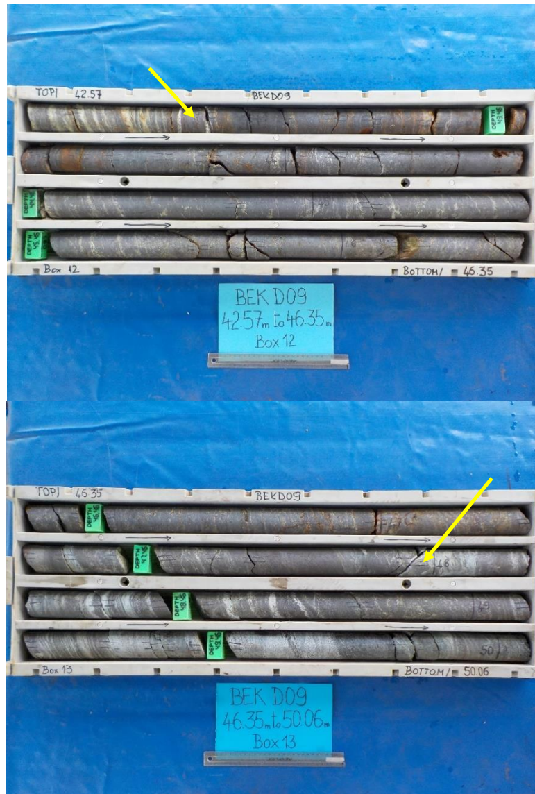
Figure 7 BEKD09; Massive iron mineralisation from 42.8m to 48.0m within a zone of more lenticular magnetite mineralisation, start and end shown within the yellow arrows.
