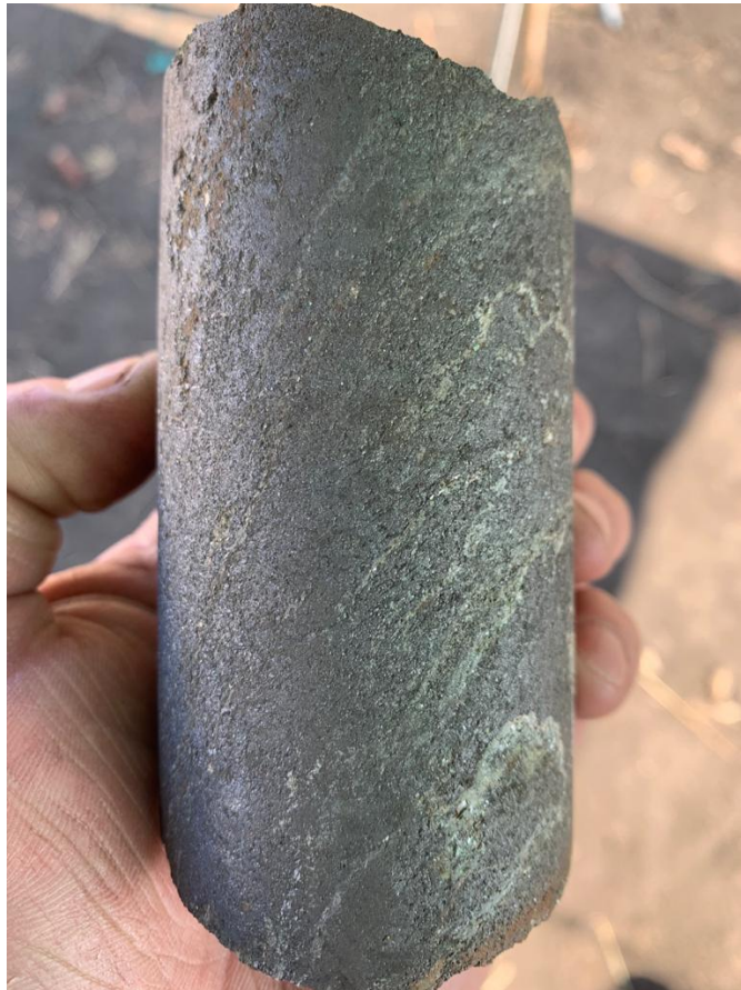
Figure 6 BEKD01 52.5m –Massive magnetite (black) with narrow layers of calc-silicate host rock (white and green)
