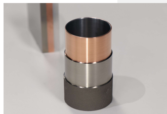
Titanium on Aluminum on Copper on Aluminum tube
