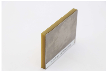
Titanium on Ultem1010 transparent polyetherimide (PEI) plastic
