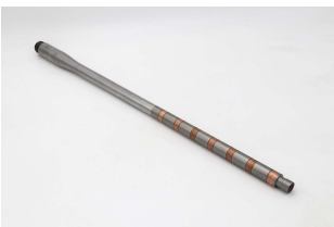
Rifle Barrel Titanium on Copper on rifle barrel mandrill
