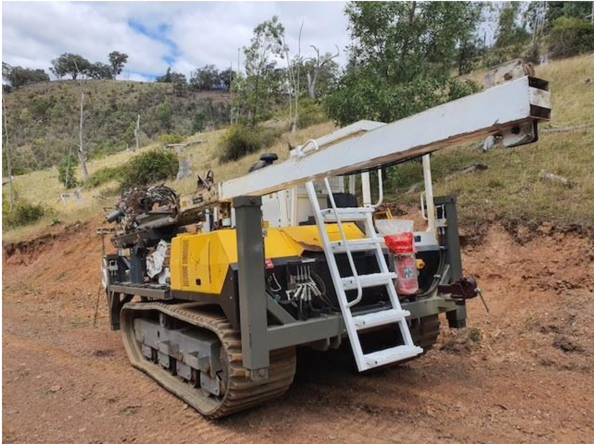
Figure 1: Diamond rig at Snowstorm Prospect, Victoria
