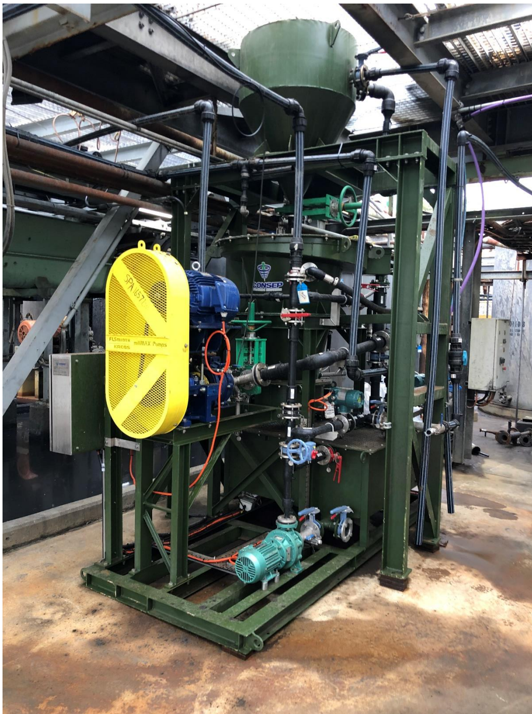
Figure 3 Consep Acacia Reactor installed at Hillgrove
