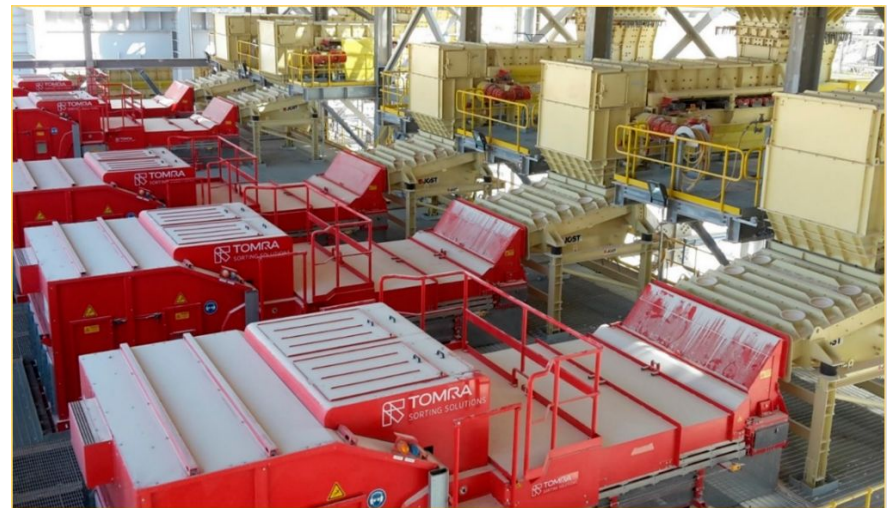
Nameplate capacity is the 1800 tons per hour XRT-based sorting plant at the Umm Wu'al phosphate mine in Saudi Arabia
