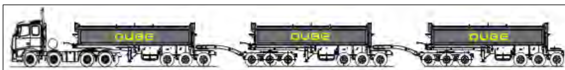
Figure 5.4 PBS Super Triple configuration
