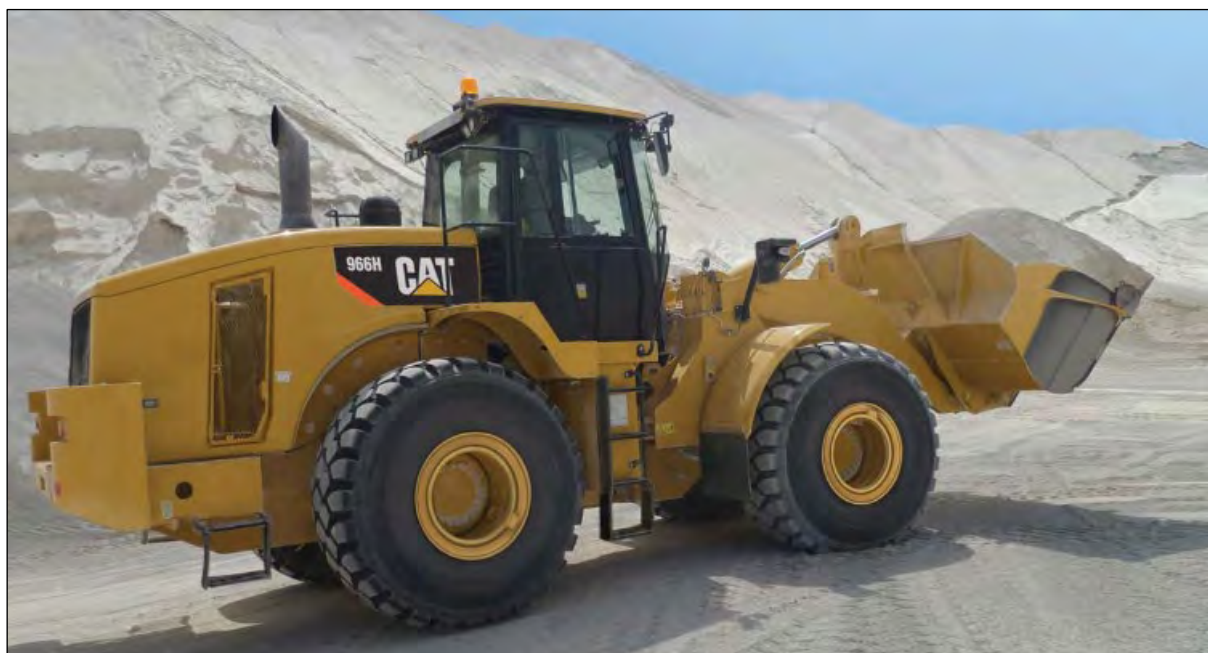
Figure 3.4 50-tonne operating weight FEL
