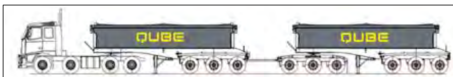
Figure 5.3 Pocket Road Train configuration
