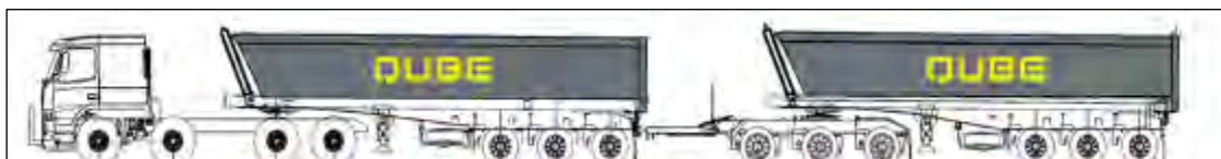
Figure 5.5 Combination End Tipper
