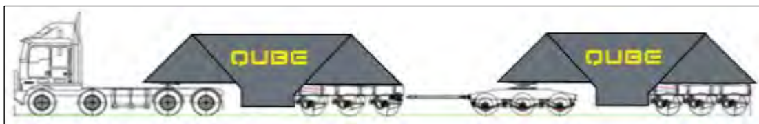
Figure 5.6 Combination Belly Dump
