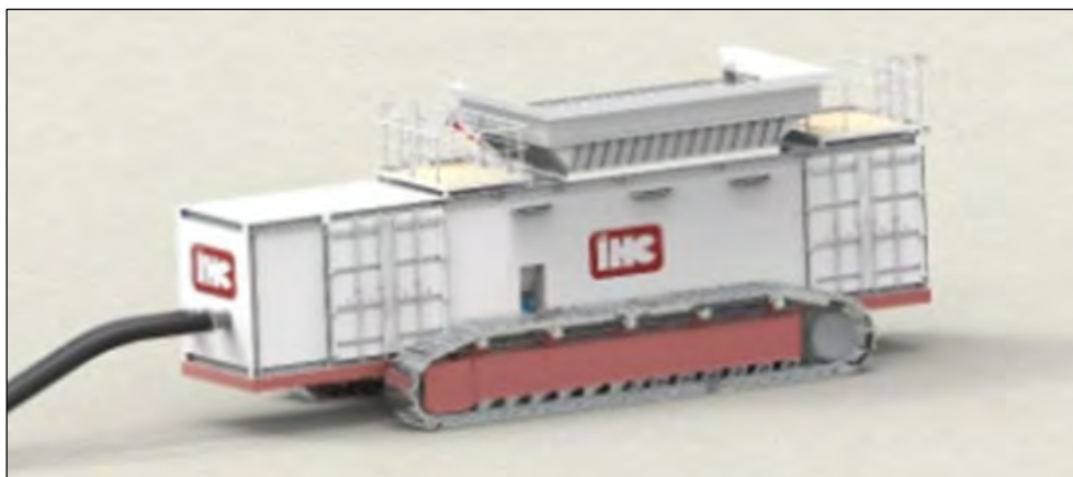
Figure 13.2 Alternative tracked containerised unit
