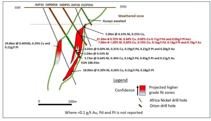
Figure 3: Geological cross-section along Section 5 showing the higher nickel grades close to surface.
