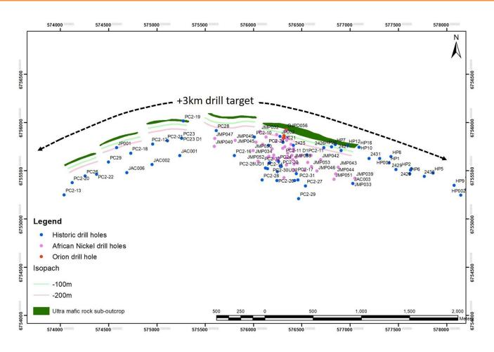
Figure 5: Map showing ultramafic sub-outcrops of the Jacomynspan Intrusive and drilling by various exploration companies.
