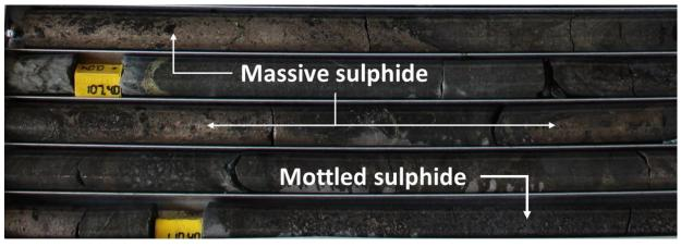
Figure 2: Massive and mottled sulphide intersected in drill hole OJPD055.
