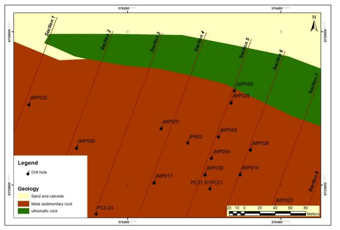
Figure 4: Map showing drill holes and section lines in the vicinity of OJPD055.
