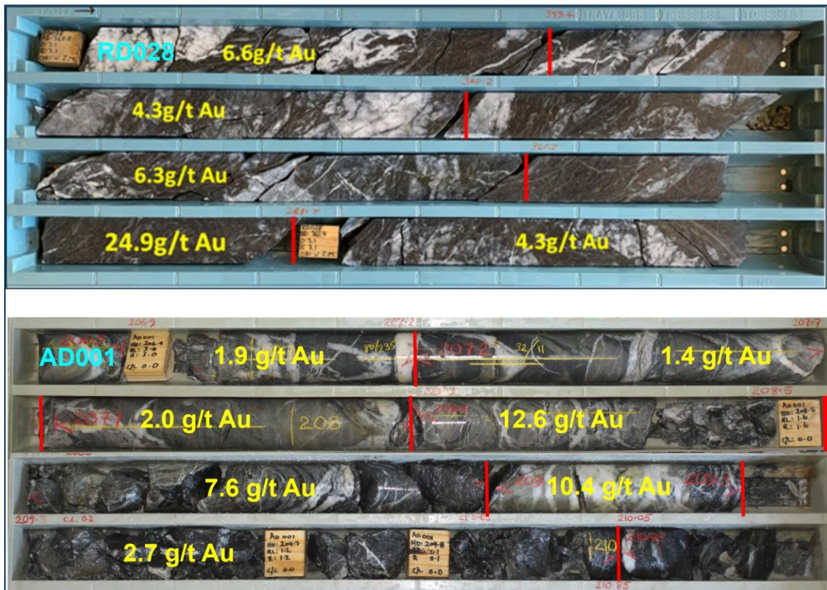
Figure 2: Examples of high-grade drill core from Resolution (upper) and Adventure (lower) prospects
