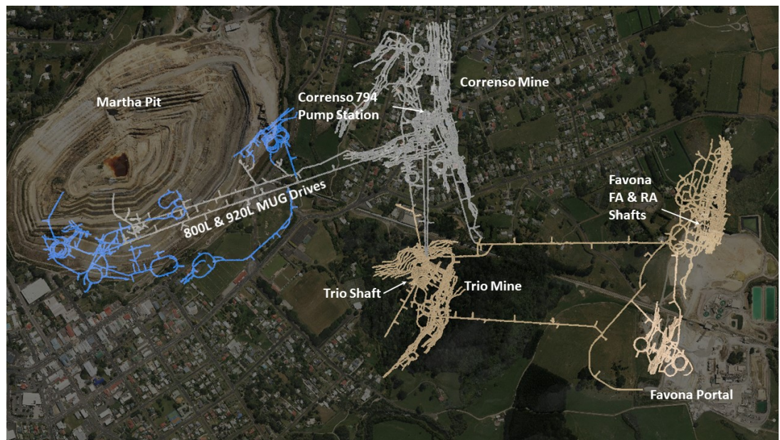
Figure 4-1: MUG Mine Access Development
