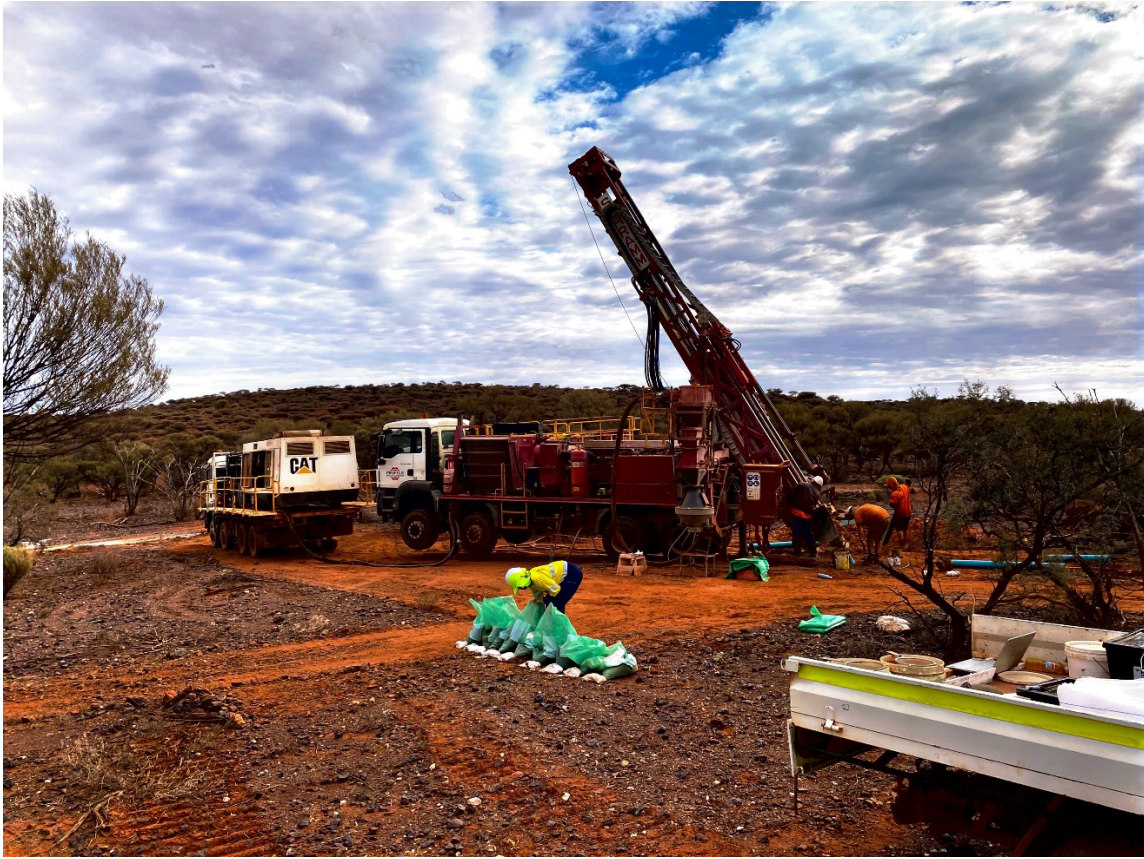
Figure 4: RC Drilling at Golden Mile's Wanghi prospect. April 2021.
