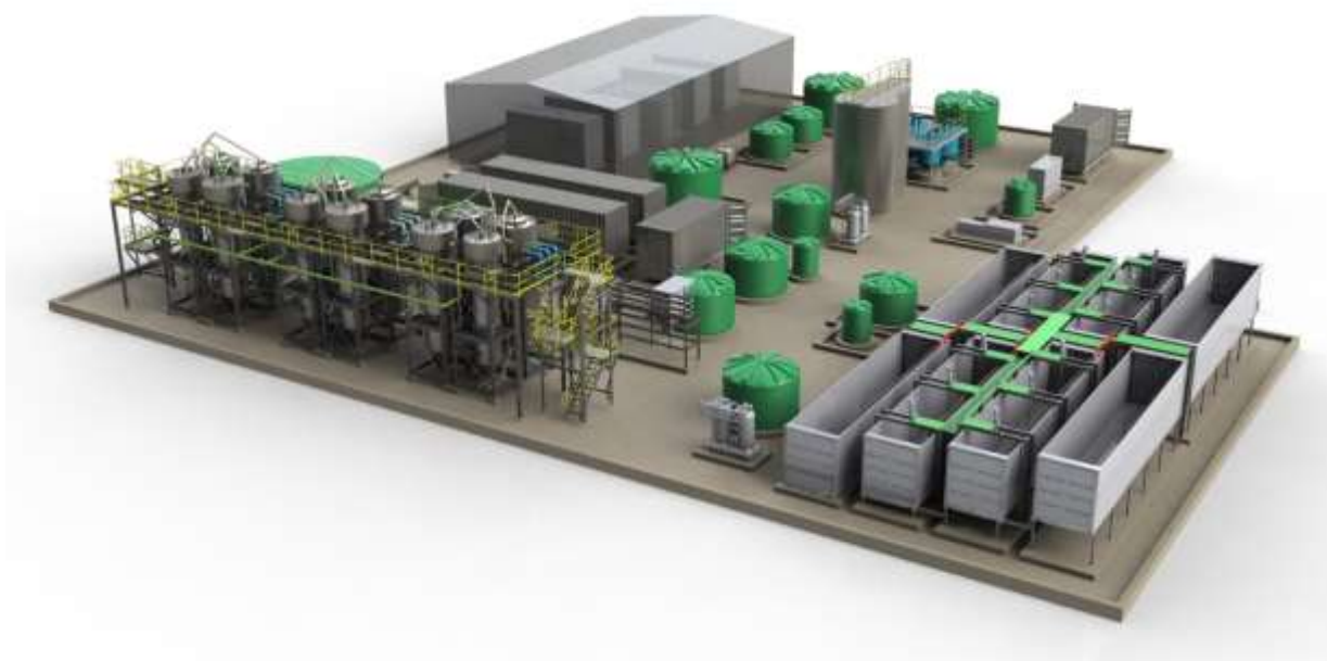
Townsville Water Purification Plant Render: The HiROx® plant combines the Company's continuous ion exchange technology with reverse osmosis and encapsulated bacteria
