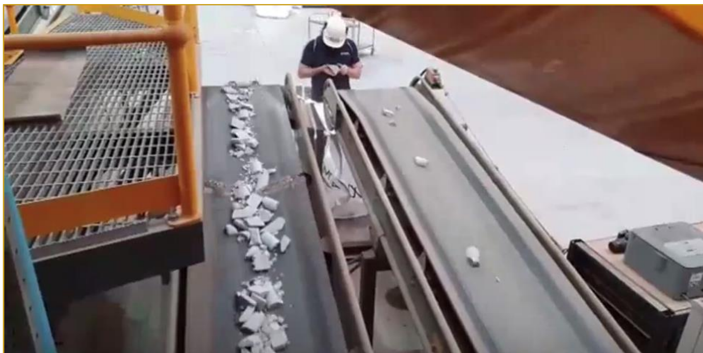
Photo 1. Korbelt Drill Core in progress on TOMRA's XRT Ore Sorter
