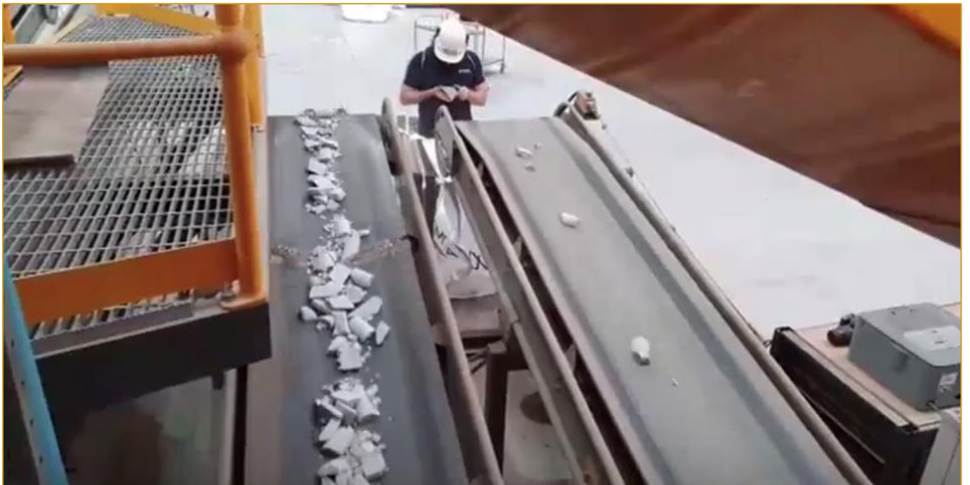
Photo 2. Korbelt Drill Core in progress on TOMRA's XRT Ore Sorter
