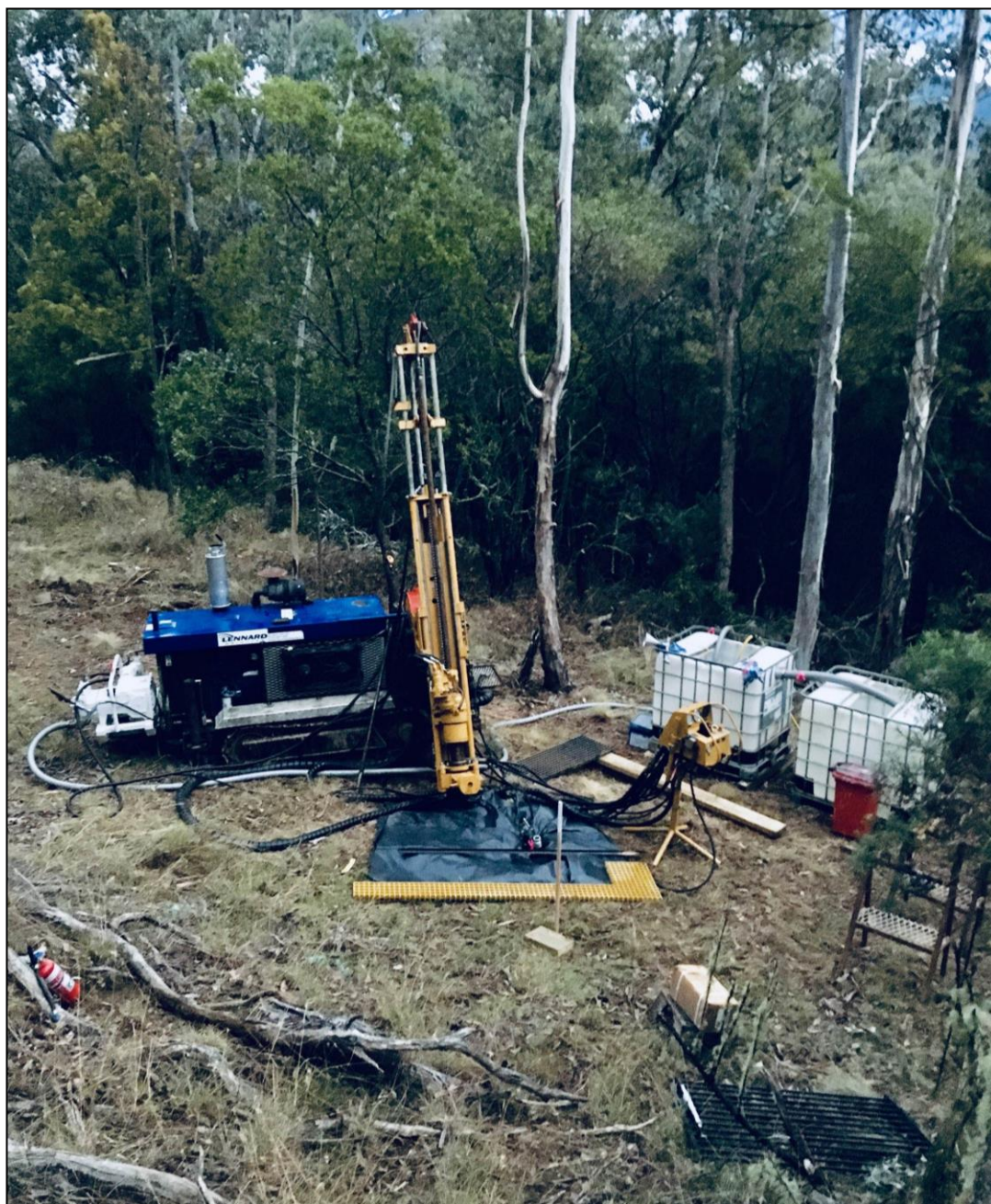
Figure 3: Dart's recently purchased Atlas Copco Diamec D262, track-mounted diamond drill rig set up at Granite Flat hole number EMPDDH01
