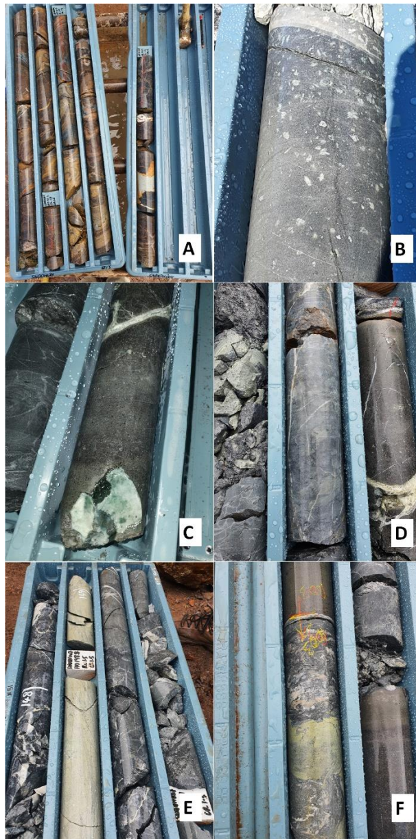
Figure 5: A) Intense carbonate (ankerite) alteration and pyritization in sediments adjacent altered dyke. B) Porphyritic 'grey' dioritic dyke. C) Chloritic alteration of mafic dyke. D) Dyke variations across several meters. Sericite altered dyke (left) and darker mafic dyke (right) displaying chill margin toward faulted sediment contact. E) Sericite altered dyke (light green) adjacent mineralised zone. F) Dyke chill margins adjacent sediment faulted contact showing sericite alteration.
