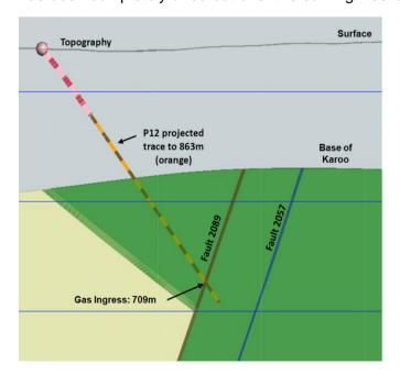
The figure above shows an approximate trajectory of the well, along with the gas ingress point. The well targeted an interpreted fault labelled 2089, to ascertain whether the fault is gas-bearing.
