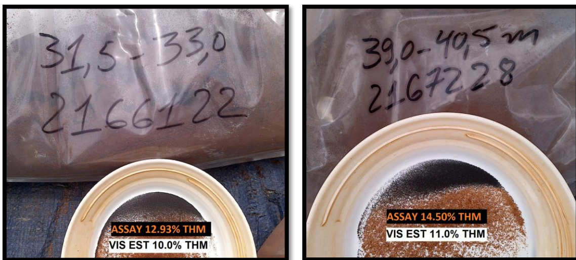
Figure 4: Images from VIS EST market update (refer ASX Announcement 06 April 2021), showing initial VIS EST and assay grades. Reference sample bags with the drill intersection, as well as the BH and sample ID (2166122 shows the 21 as drill year, 661 as the BH ID and 22 as the sample number).
