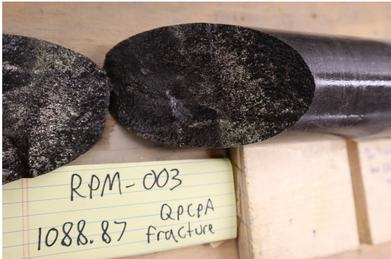
Figure 8: RPM-003 Pyrite-Chalcopyrite mineralisation in hornfels
