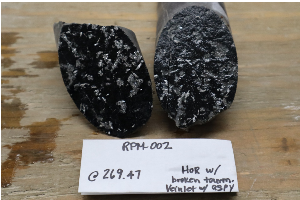
Figure 7: RPM-001 - Arsenopyrite-tourmaline veinlet in hornfels
