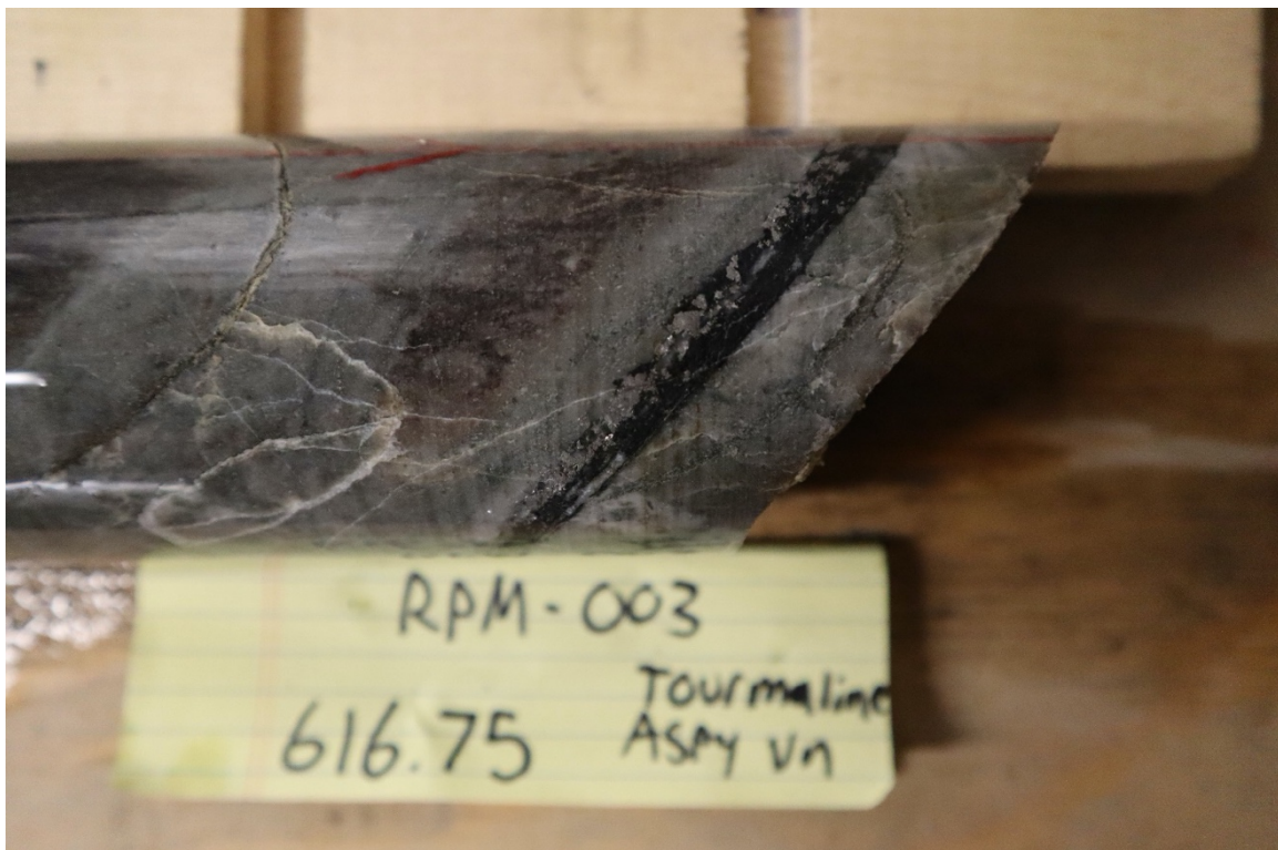
Figure 9: RPM-003 – Tourmaline-Arsenopyrite vein in hornfels
