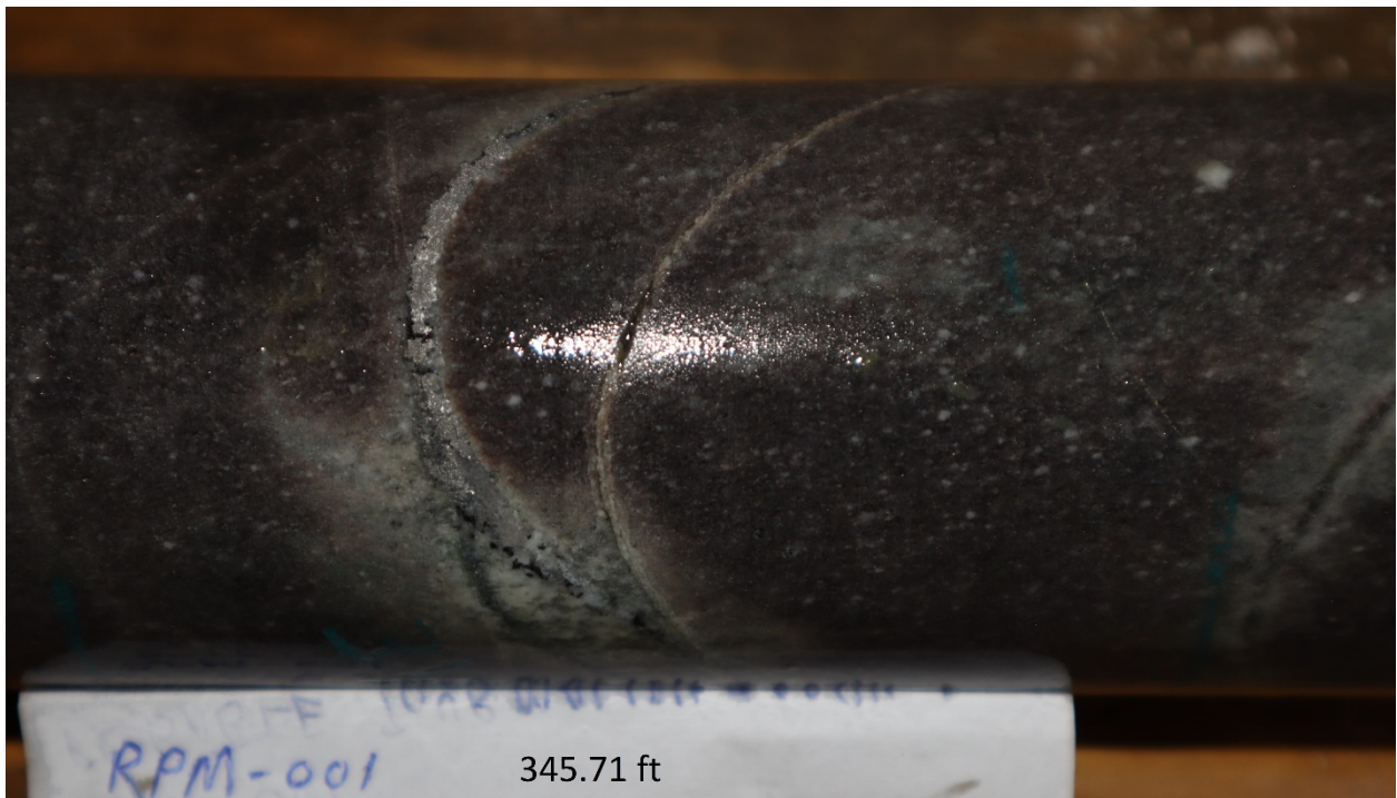
Figure 5: RPM-001 - Arsenopyrite veinlet in hornfels
