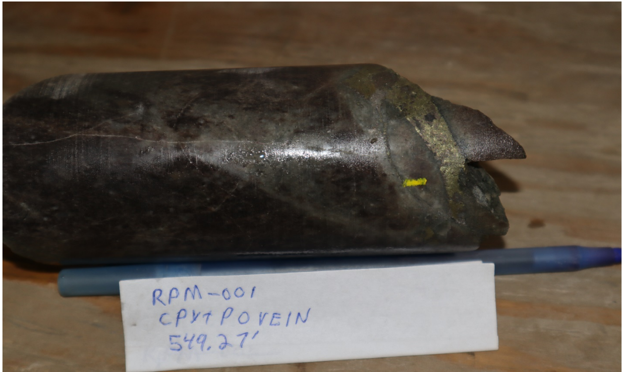
Figure 6: RPM-001 - Chalcopyrite-pyrrhotite vein in hornfels
