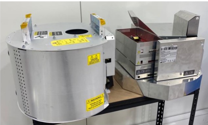
Current (left) and future (right) Generators for the Rover range of Mobile DR x-ray products – future generator delivering four times more power
