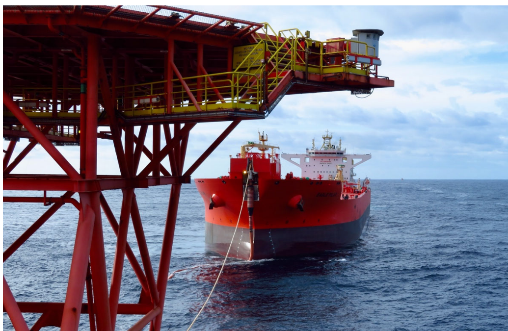
Preparations to offload Baúna crude from the Baúna Floating Production, Storage and Offtake vessel (FPSO), Cidade de Itajaí, to the Shell tanker, Eagle Pilar
