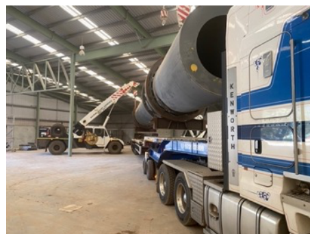
Photo (left): The driver reversing the specialised extendable trailer under the kiln.
