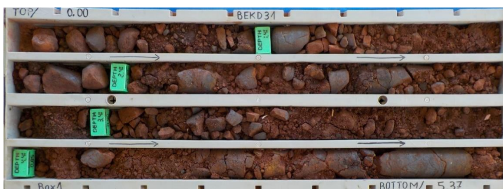
BEKD32 - 0 to 4.18m Weathered Massive Iron Mineralisation
