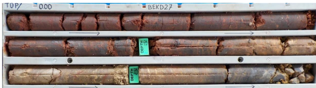
BEKD28 - 0 to 3.2m Weathered Massive Iron Mineralisation
