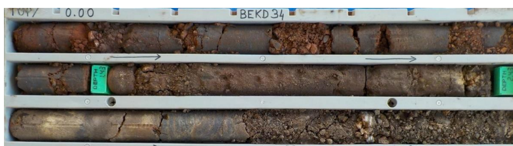
BEKD34 - 0 to 3m Weathered Massive Iron Mineralisation
