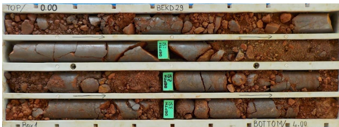
BEKD30 - 0 to 3.9m Weathered Massive Iron Mineralisation
