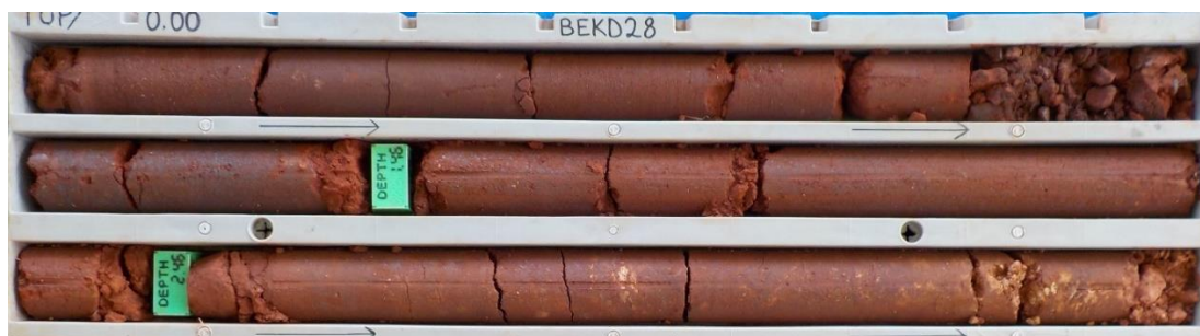
BEKD29 - 0 to 4m Weathered Massive Iron Mineralisation
