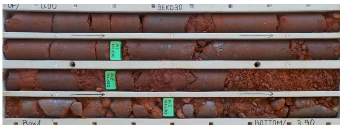
BEKD30 - 0 to 3.9m Weathered Massive Iron Mineralisation
