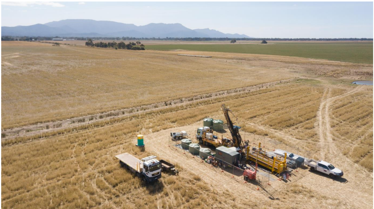
Figure 4: Diamond core drilling at Morning Bill during March 2021.
