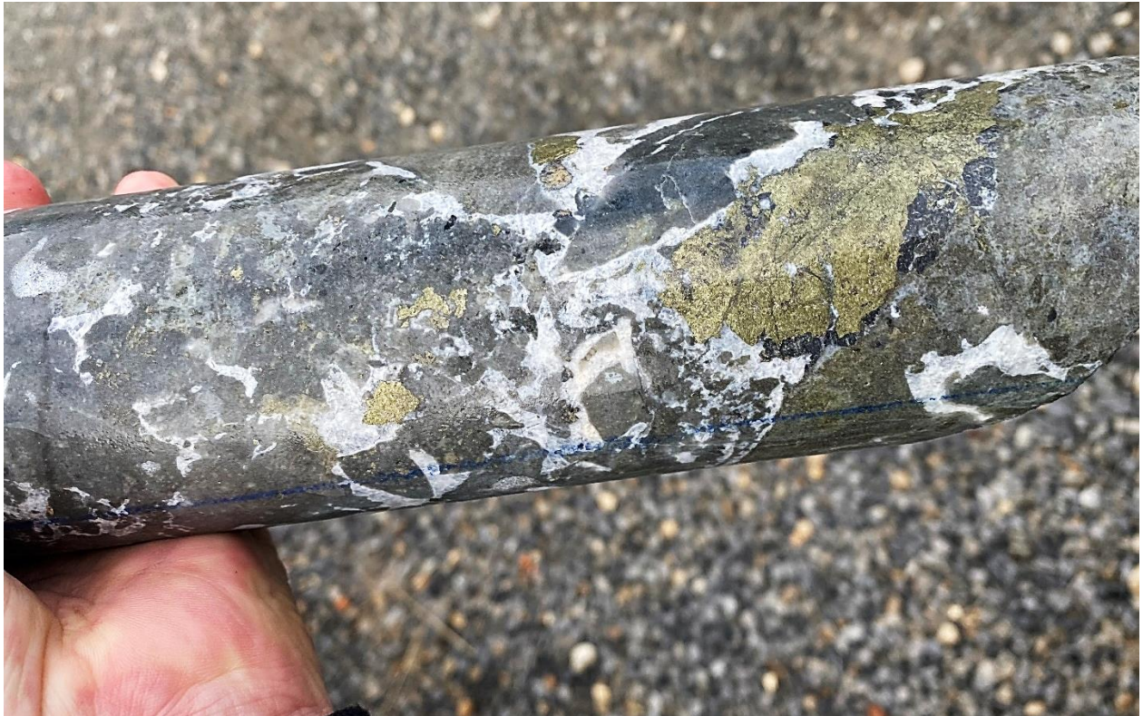
Figure 5: Copper-rich drill core assaying up to 1.2% Cu from approximately 215m in GDD003.
