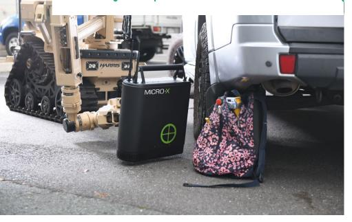
Robotic deployed, remotely viewed, high resolution x-ray imaging
