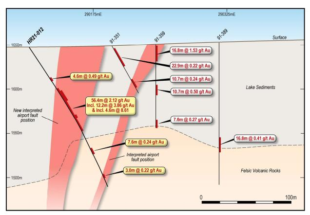
*Figure 2:* Cross section view (see Figure 1 for location) highlighting the drilling results from hole HR21-012 relative to the surrounding historical drilling information.
