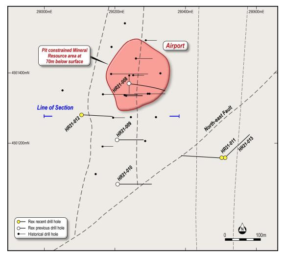
**Figure 1:** Plan view of the drill holes from the Airport area relative to the existing Mineral Resource estimate of 60Koz (see ASX release 23 March 2021) – dashed lines represent interpreted structures based off recently acquired geophysical 3D Induce Polarisation (IP) data.
