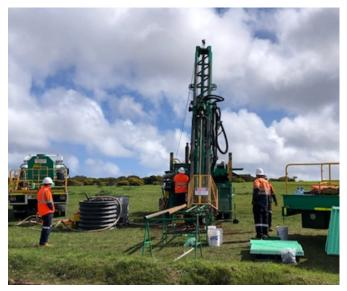
Figure 1: Diamond drill rig on site at Uley
