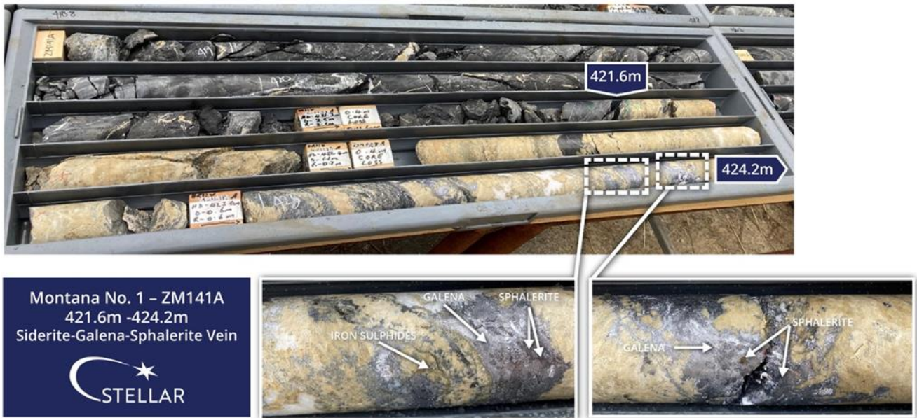
Figure 6 - Montana No. 1 Drillhole ZM141A, Fissure Vein from 421.6m to 424.2m with visual sulphide galena and sphalerite mineralisation containing, lead, zinc, silver, copper and tin
