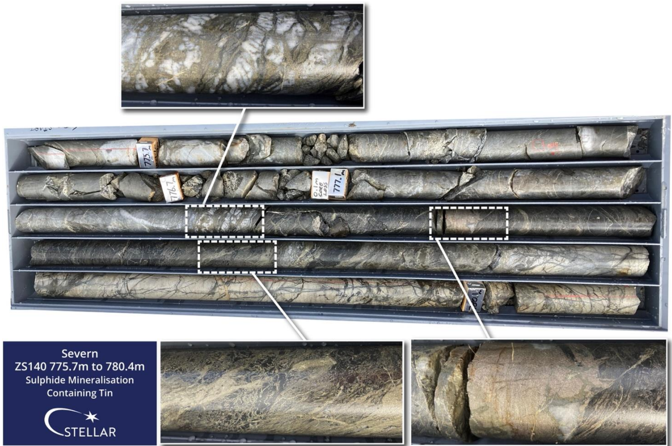
Figure 3 - Severn Drillhole ZS140, Typical example (775.7m – 780.4m) of sulphide mineralisation containing tin
