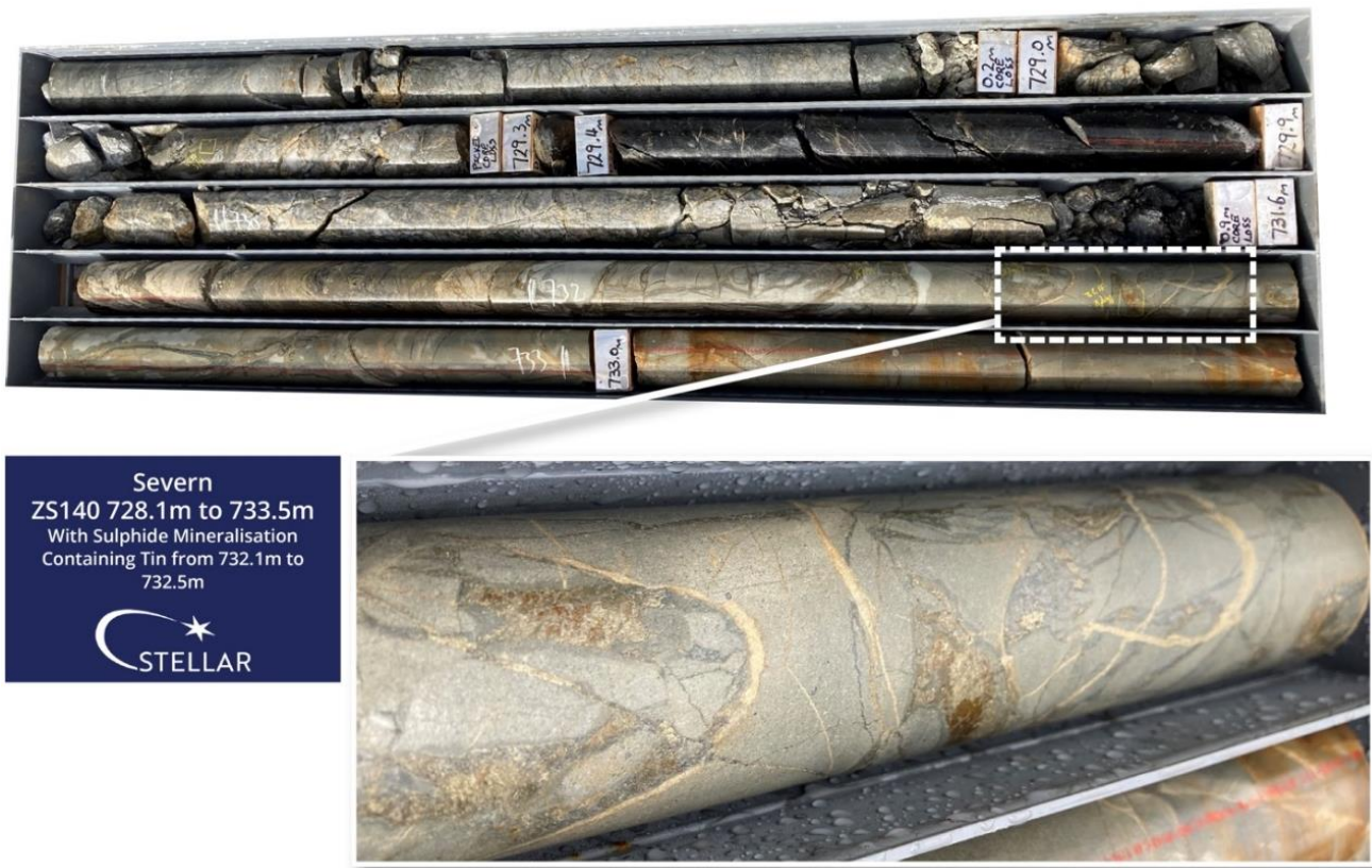
Figure 2- Severn Drillhole ZS140, Typical example (732.1m to 732.5m) of sulphide mineralisation containing tin
