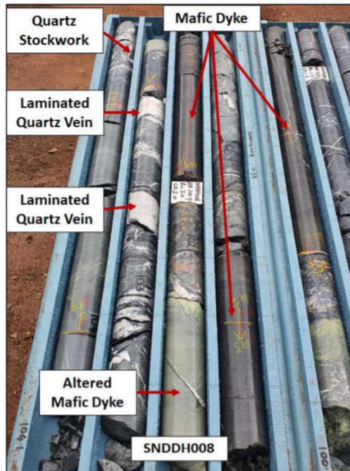
Figure 5. Mineralised quartz-veins intimately associated with mafic intrusions.
