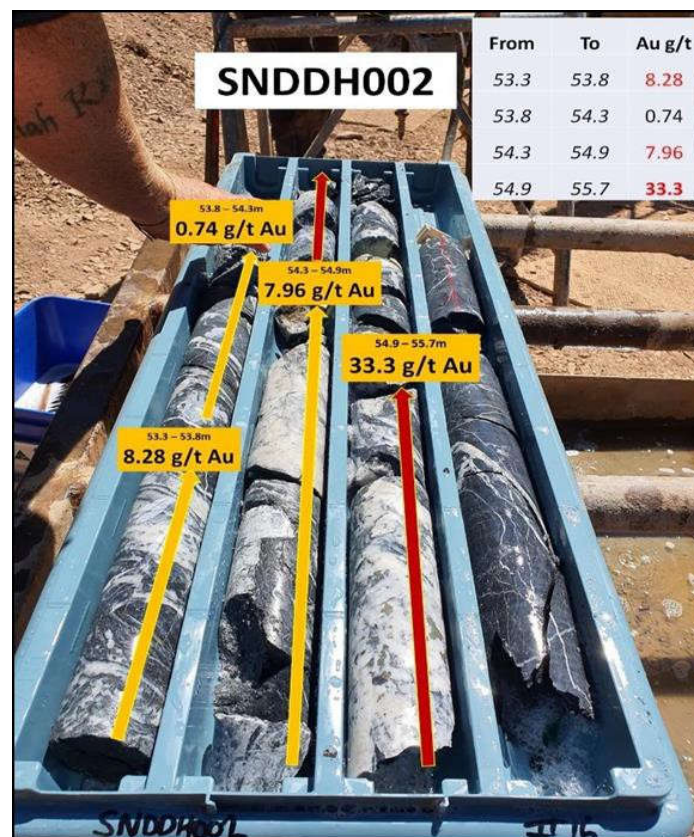
Figure 3. SNDDH002 diamond core with mineralised interval.
