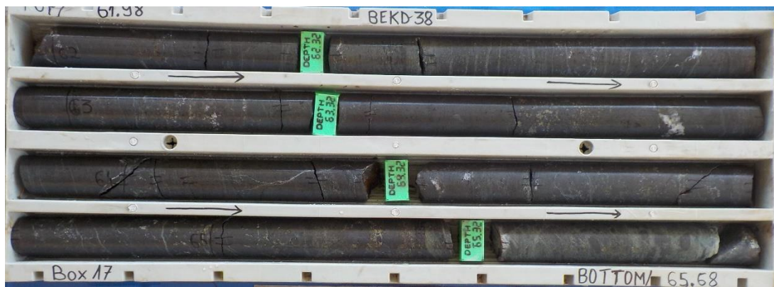
BEKD38 - 73.32 to 77.42m Massive Iron Mineralisation
