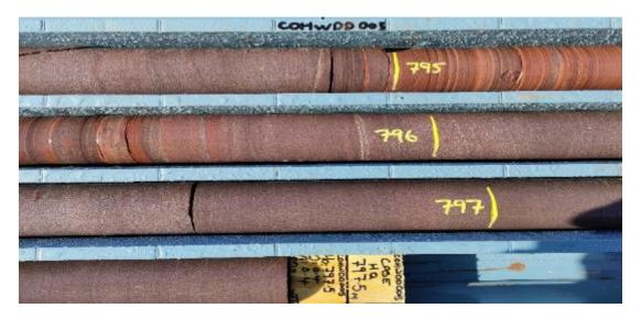
Figure 1: Drill core from HWDD05 (797.5m) showing typical Pandurra Formation.
