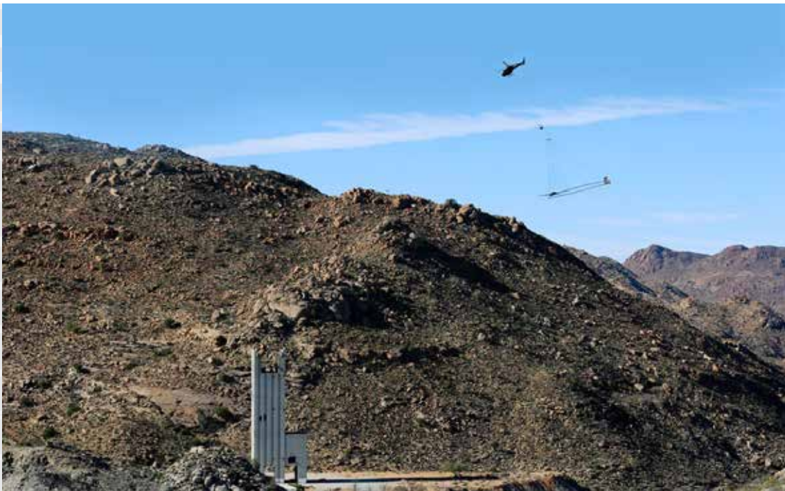
FIGURE 13: SKYTEM™ FLY-OVER AT CAROLUSBERG MINE (DEFUNCT SHAFT IN FOREGROUND).
