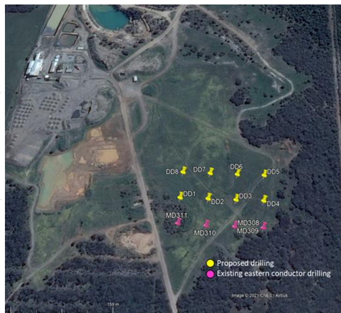
Figure 2: Eastern Conductor Drillhole Locations
