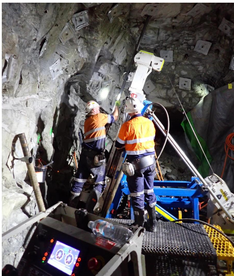
Photo 1: Deepcore underground drill rig drilling the first exploration hole into the Gap Zone on Ring 3 at the Morning Star Gold Mine.
