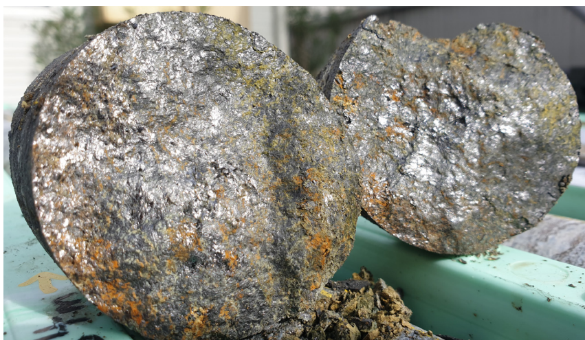
Figure 7: Typical presentation of coarse flake from drill hole MD705 at a depth of 54m.
