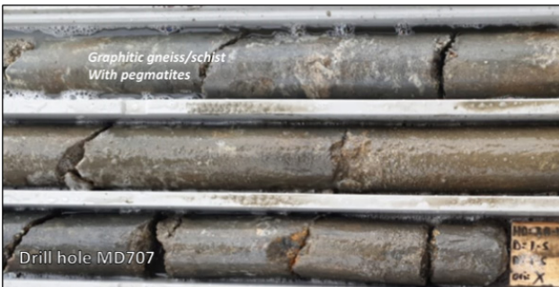
Figure 3: MD707, close-up of mineralisation and alteration. 35.4 to 38.1m estimated visually as +20% TGC
