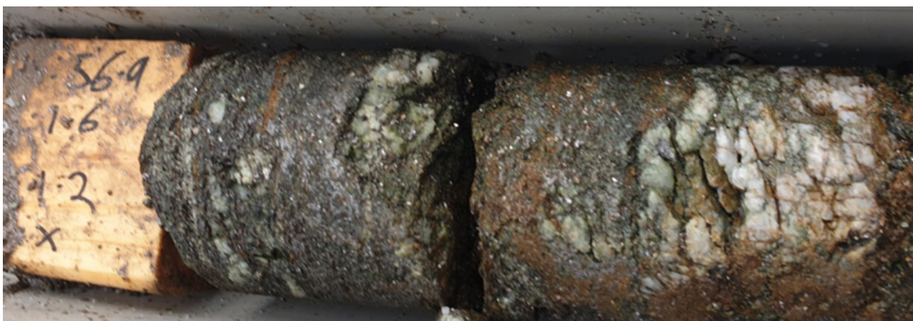
Figure 6: Example of Coarser flake graphite associated with pegmatite from drill hole MD708 at a depth of 56.9m.
