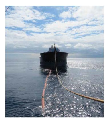
Offloading from the Baúna Floating Production, Storage and Offtake vessel (FPSO), Cidade de Itajaí, to Shell tanker
